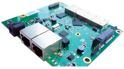
WPJ342 is a capable and reliable wireless embedded board based on the Qualcomm Atheros AR9342 CPU. It features a 560MHz network processor and integrates a 2x2 internal on-board radio and 1 miniPCle slot that supports 802.11n radio. Embedded with 64MB memory and 16MB Flash, WPJ342 provides the ideal platform for any applications. WPJ342 has integrated Power over Ethernet (PoE) features that allows WPJ342 to be used in areas where power outlets are not readily available.
